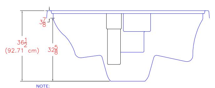
Dimensional tolerances are as follows due to variations in manufacturing: Length / Width / Height(s): +/- 3/8" Height Variance (side to side): +/-1/4"
