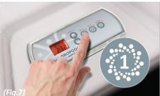
to high or pump 2 icon to turn on or off (Fig.7). After pressing the buttons please make sure water is circulating through the jets. If there is no circulation, you may have an air lock. Please refer to Owner's Manual to clear the air lock.
