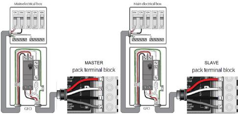
240 V (4 wires) Refer to wiring diagram in the enclosure box lid for more information.
